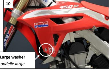
Fix the plastic cover with Tbhc 6x16mm + Large washer
